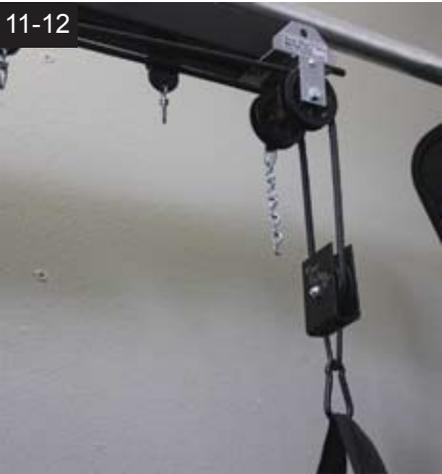
12) Pull rope through the remaining bolt bracket on the master carrier, tighten bolts and tie a knot.
