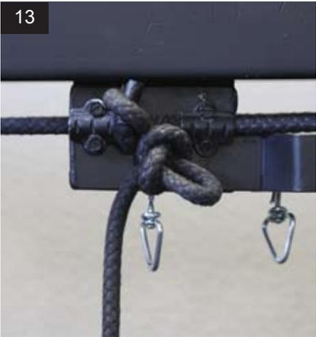
13) Fly truss up to trim height, measure excess rope between live end pulley and floor pulley with sand bag hanging one foot off ground.
