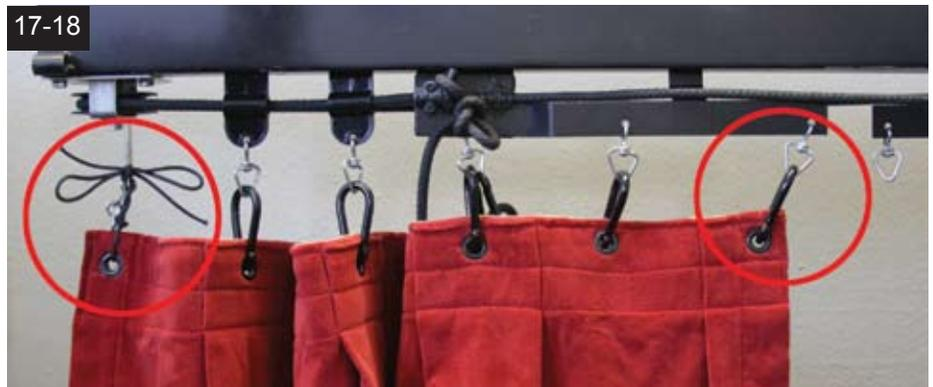
18) Fly to trim height and test. Adjust as needed by loosening end bolt bracket and retying knot to adjust rope length as needed.
