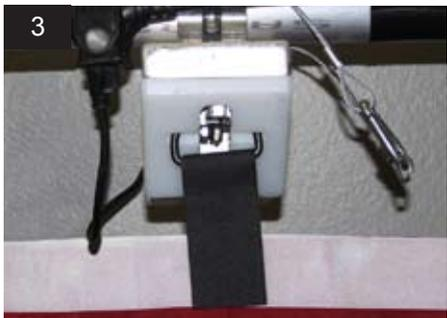
3) Next, position your D-rings on the drape using the Velcro tabs to align with the solenoid heads. Always use the Velcro style D-ring to drape connectors provided. Attach the D-rings to the heads by pushing the ring into the slot on the underside. You will hear the mechanism click when the ring is locked in place.
