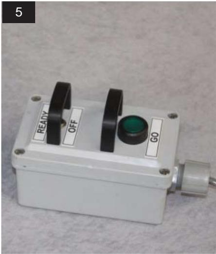
5) The controller cable will connect to the port labeled "REMOTE" on the power supply. Flip the switch on the controller to the ready position to display a green light on the GO button, and then push the lit button to release the Kabu-KEY! Kabuki.
