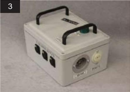
3) From the female receptacle on the first head in a group, run a XLR cable down to the power supply provided and connect to one of the ports labeled "V3 SOLENOID OUTPUTS." Use the provided twistlock cable to connect from the port labeled "120 VAC" to your power source (input voltage range from 100 to 240 V 50/60 hz ).
