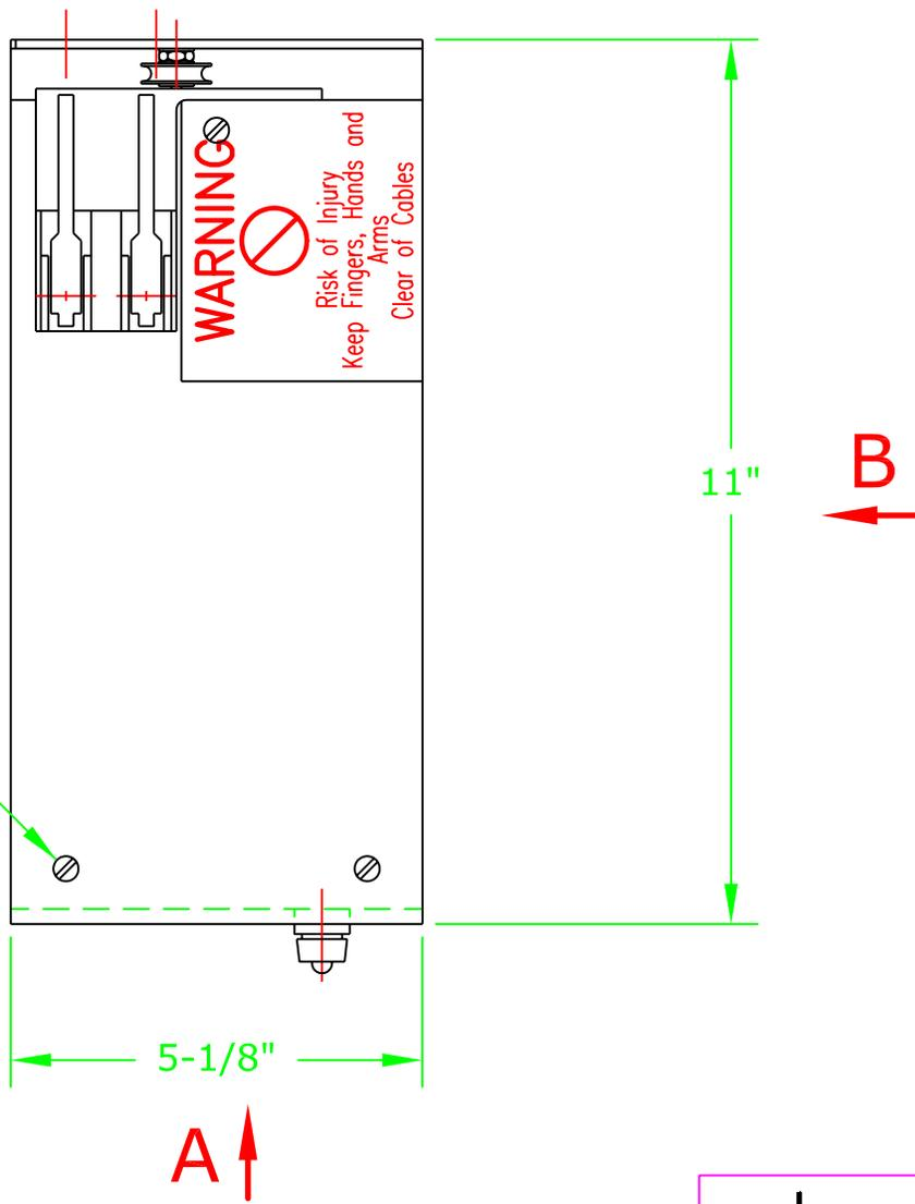
REMOVE SCREWS (7 TOTAL) TO REMOVE COVER
